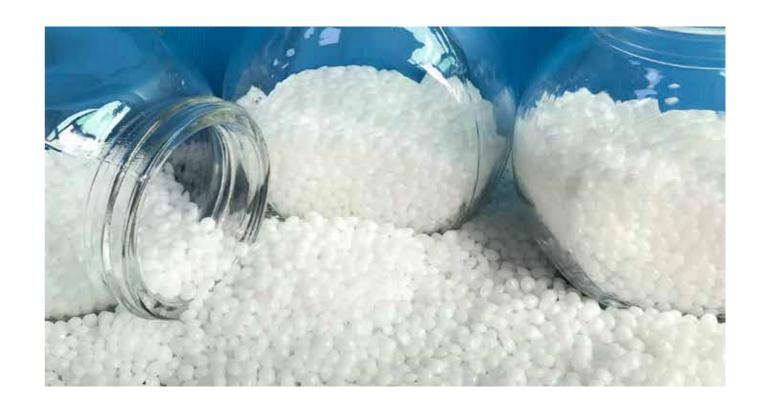
Polyacetals or commonly known as POM is used in precision parts requiring high stiffness, low friction, and excellent dimensional stability. Typical applications for injection-molded POM include high-performance engineering components such as small gear wheels, valves, bearings, zippers, fasteners and lock systems. The material is widely used in the automotive and consumer electronics.
